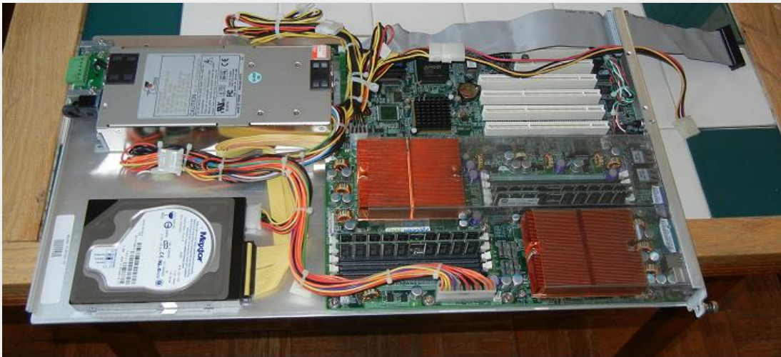
A single slide-in blade from the UHSSC Competition System
